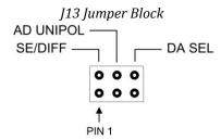
Jumper LabelConfiguration FunctionSE/DIFFA/D single-ended/differential selection.AD UNIPOLA/D unipolar/bipolar selection.DA SELD/A unipolar/bipolar selection.
